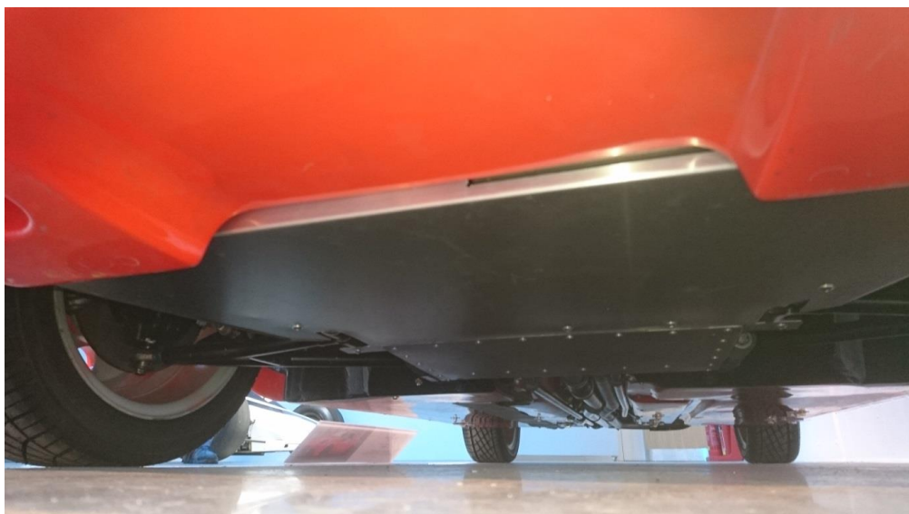
Front undertray as fitted to the car in 2017 - Author's photo
