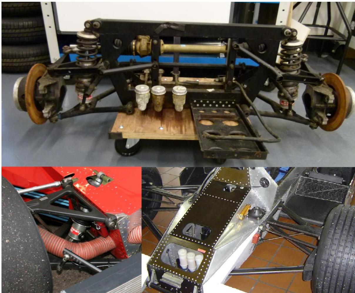
Top: Midas-Alfa front suspension assembly
