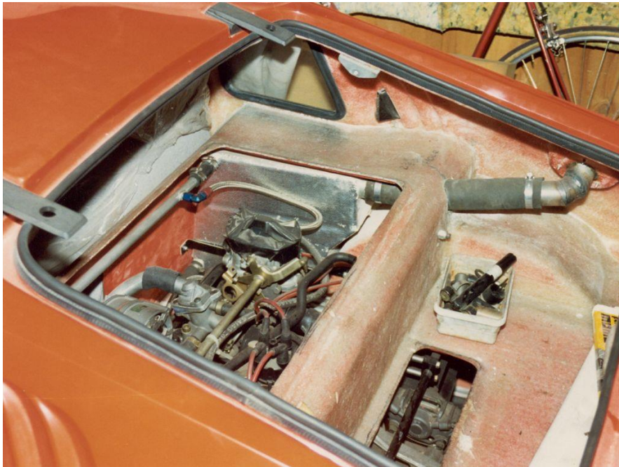
Photo courtesy of Hugh Brodie - Alfa engine mounted in modified Midas monocoque.
